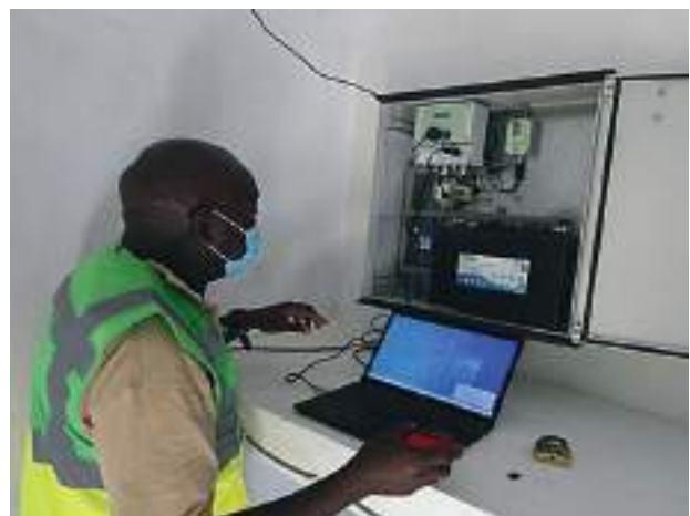
WRA Technical Officer demonstrating how data is downloaded from the telemetric station into the computer.
