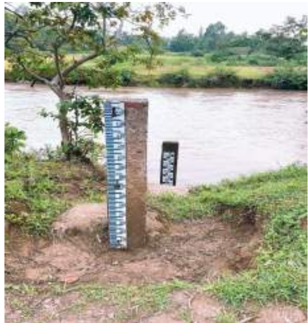
Manual Gauging Plates at Nzoia River in Webuye to measure the flows of the river.
