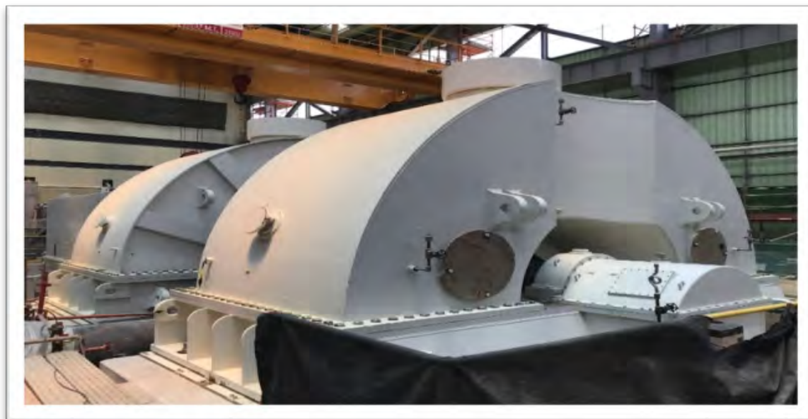
Figure 3-2: 83.3MW Olkaria 1 Unit 6 - Steam Turbine and Generator
